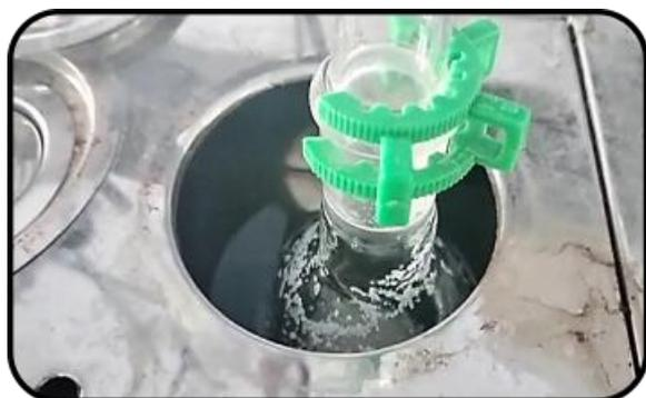
**Step (iii): The mixture kept in water bath about 78°C for 30 minutes**
